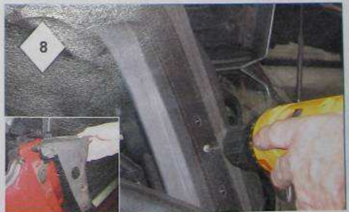
Remove rivets from B-pillar retainer. Remove B-pillar cap weather seal.
