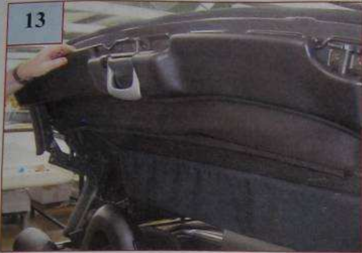
Install the header bow cover.
