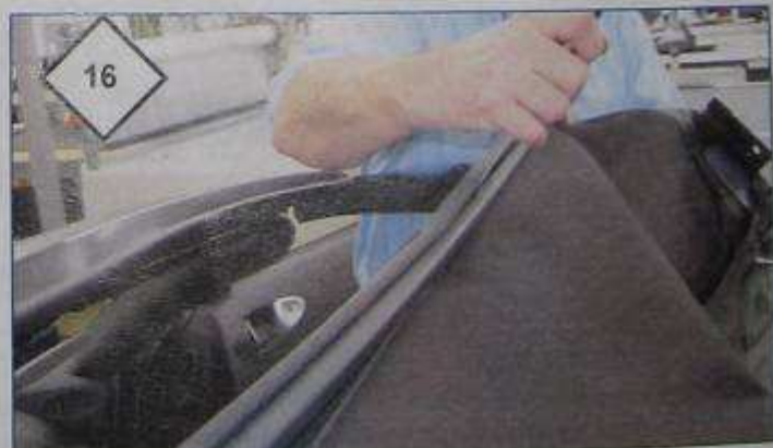
Use a putty knife to release the 2-bow listing.
