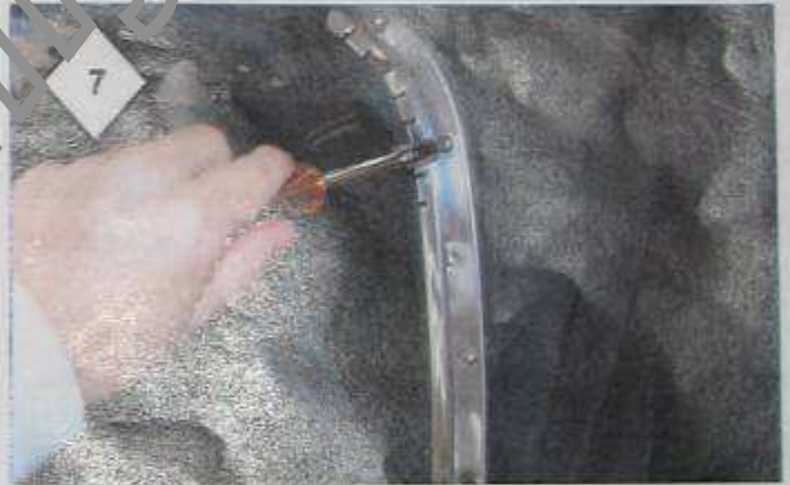
Remove rear-side weather seal retainers.
