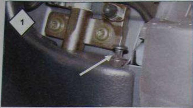
Remove pins from the header bow cover.
