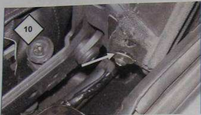
Remove screw and washer from bottom of the B-pillar.
