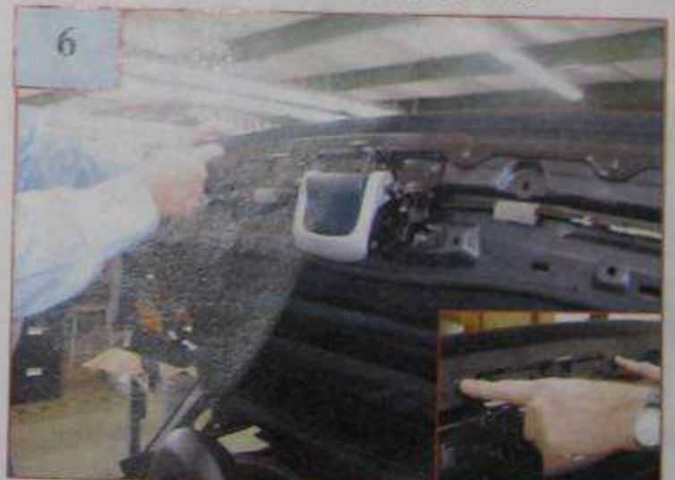
6 Secure inside center part to header with tape, making sure holes are aligned. Then attach header retainer with 8 screws.
