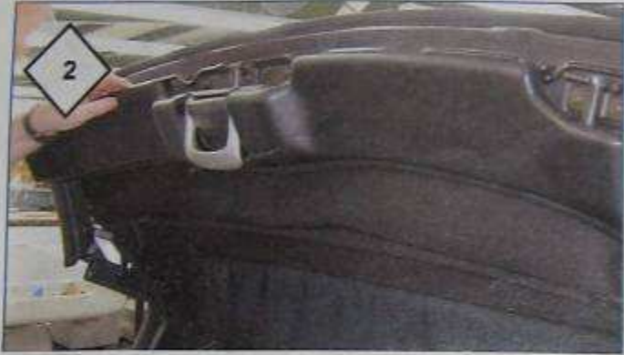
Remove the header bow cover.
