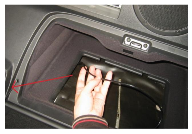
From there, feed the cable through the centre console as indicated by the arrow and the picture below
