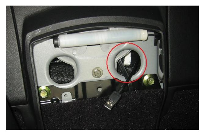
Using zip ties and common sense, route the cable along the existing wiring:
