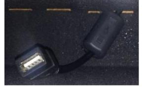
On the outside, I used Zip ties. The loop is to protect the cable from strain should there be excessive pull from the inside.
