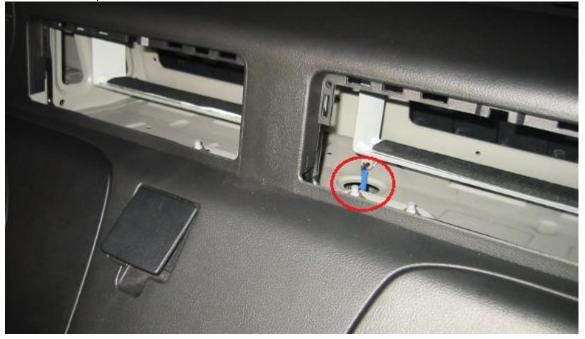
Once you get the cable through the hole circled above, you'll need to grab it from the bottom of the glovebox, to access this you just need to pop out the plastic cover with a trim removal tool or a screwdriver.
