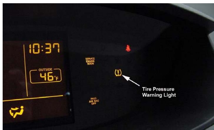
Picture 6: Low Pressure Warning Light Shown Illuminated
