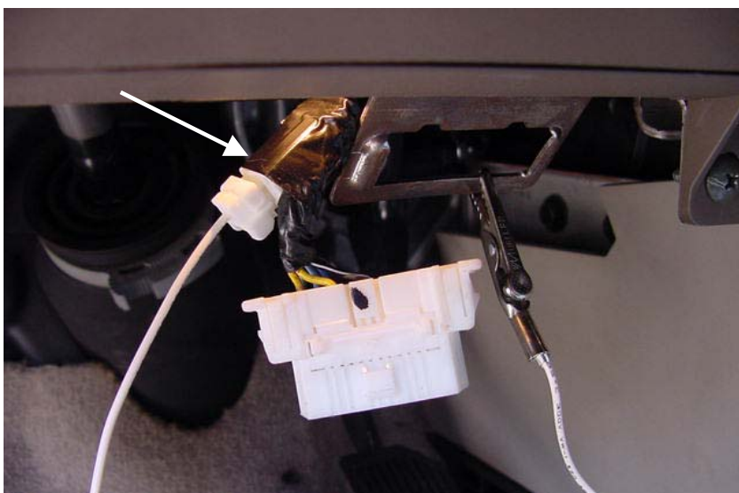
Picture 3: Special connector plug grounded to mounting bracket.
