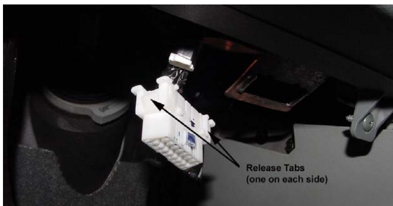
Picture 2: Release tabs on DLC.
