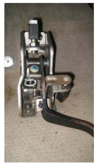
CAUTION!!! - The Clutch Assist Spring Mechanism is powerful and due to its over-center cam design it will snap violently like a mouse trap in either direction once you reach the tripping point.
