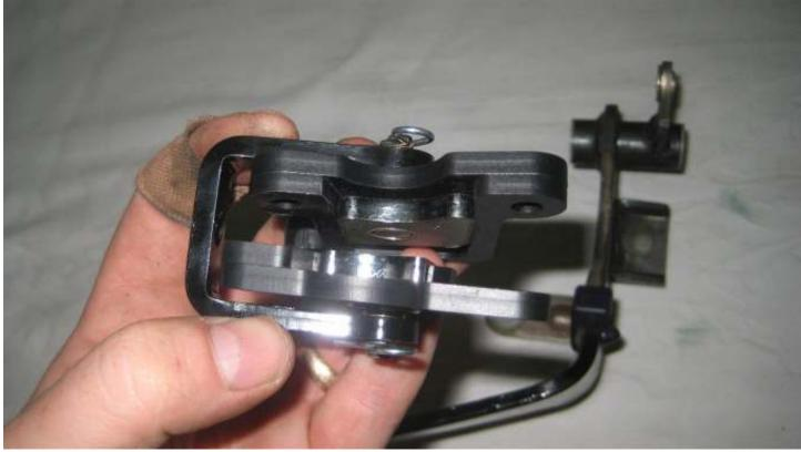
. You will need to guide the assembly in place around the switch pad mounts in order to get it fully seated against the pivot tube at the top.
