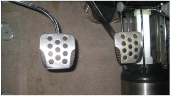
Once you're satisfied with the initial position of the clutch pedal go back and adjust the upper switch so that it too gets just depressed by the pedal while fully at rest but does not bottom out the switch and hold the clutch pedal from returning all the way up.
