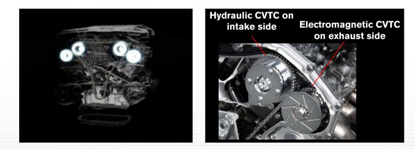
**CVTC** intake and exhaust controls on both sides
