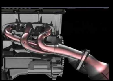
Equal length exhaust manifold
