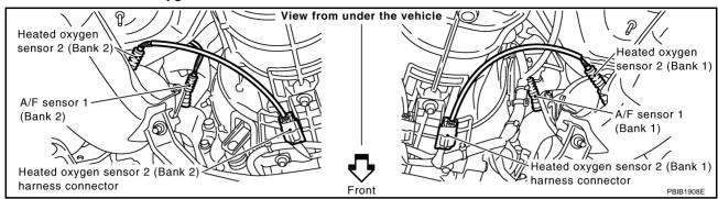
3. Check harness continuity between HO2S2 terminal 4 and ECM terminal 78. Refer to Wiring Diagram.
