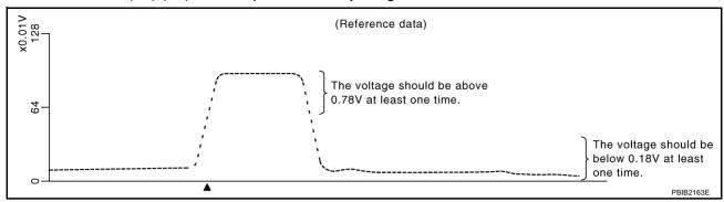
"HO2S2 (B1)/(B2)" should be above 0.78V at least once when the "FUEL INJECTION" is +25%. "HO2S2 (B1)/(B2)" should be below 0.18V at least once when the "FUEL INJECTION" is -25%.
