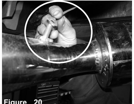
Figure 20 Connect the grounding wire located at the rear of the vehicle to the welded bolt on the driverside muffler piping.
