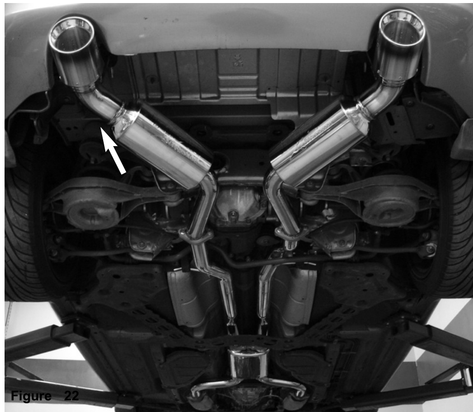
Figure 22 Congratulations! You have just completed the installation of the Injen cat-back exhaust system. Periodically, check the fitment of the exhaust system, the exhaust should always continue to hang in the same position.
