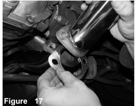
Figure 17 Place a 60mm gasket in between the rear muffler and mid-pipe on both left and right side.
