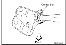
3. Tighten both nut of the right and left side of center bolt.
