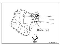
3. Remove tower bar fixing bolts and nuts, and remove tower bar from vehicle with power tool.
