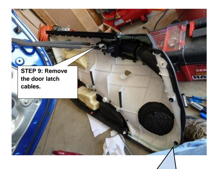
After you have removed the door panel, check the steel door and make sure none of the plastic trees stayed in the door. If they did, just remove them and reinstall into the door panel. The door panel will never reinstall correctly with the trees still stuck in the door.
