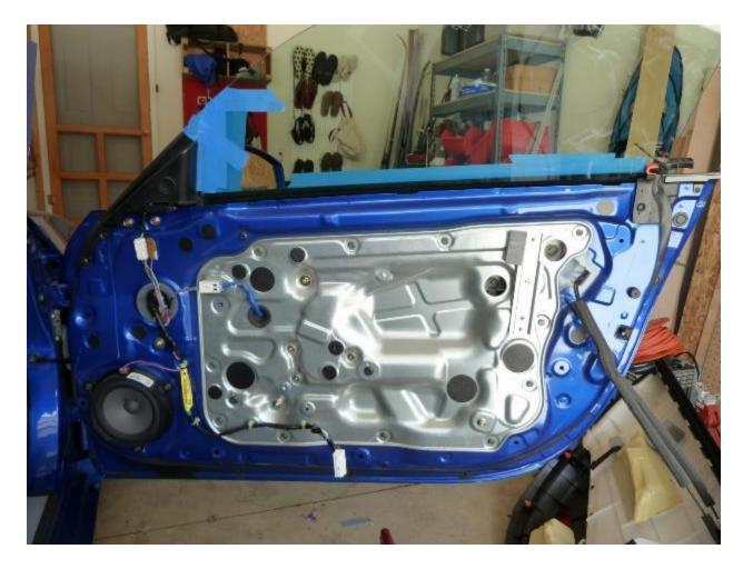
Only AFTER you have reinstalled all fasteners can you remove the clamps and tape on the window. Do not install the final door panel until after you perform the motor reset procedure.
